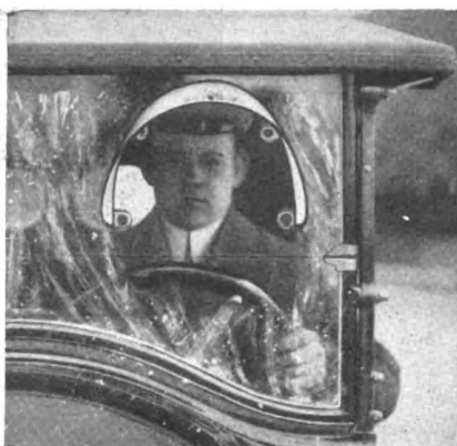
How the U-Can-C shield keeps the space in front of the driver clear
